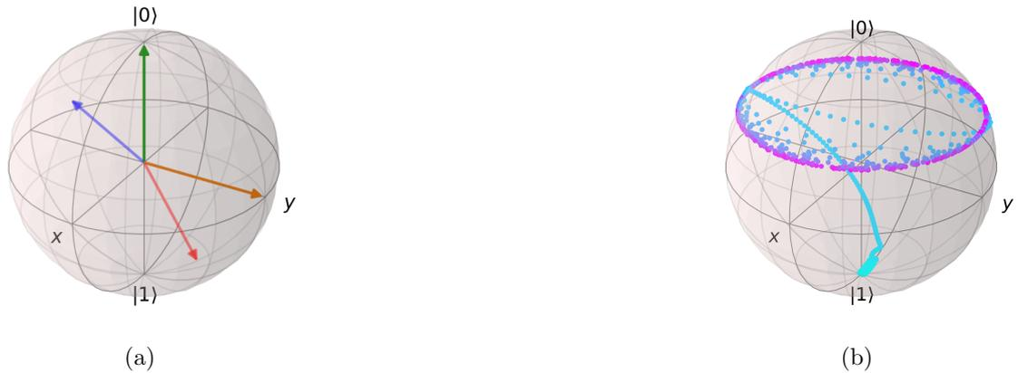
FIGURE 1.2 – (a) a graphical representation of a qubit on a Bloch sphere. (b) Landau–Zener evolution of a two-level system represented on the Bloch sphere. Figures generated using QuTip package (JOHANSSON *et al.*, 2012; JOHANSSON *et al.*, 2013).
